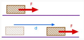
When force and displacement are in the same direction, a simple work equation is W = Fd
