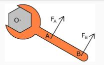
Torque is a vector - its direction is along the chosen axis of rotation, and can be determined by the righthand rule:
