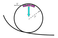
Non-uniform circular motion may also have tangential acceleration - a component of **a** parallel to the velocity (tangent to the circle)
