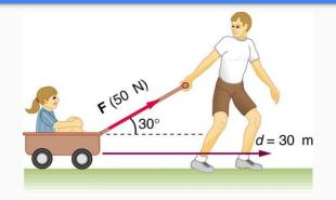
When **F** and  $\Delta d$  are not parallel, we can use components to calculate the work done. For this wagon:
