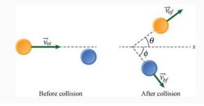
In such a collision, conservation of momentum still applies: the total momentum vector for the system before the collision must equal the total momentum vector after the collision.
