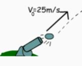
$v_{0x} = v_0 \cos(\theta)$   $v_{0y} = v_0 \sin(\theta)$ So now we can write:  $v_y = v_0 \sin(\theta) + a_y t$   $\Delta y = v_0 \sin(\theta) t + .5a_y t^2$  $\Delta x = v_0 \cos(\theta) t$
